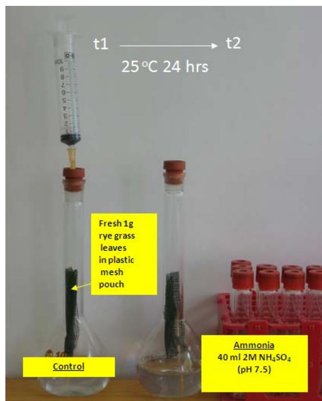
Figure 1: Experimental set up to detect  $\text{N}_2\text{O}$  emissions from detached leaves and detached leaves exposed to high ammonia ( $\text{NH}_3$ ) environments.
