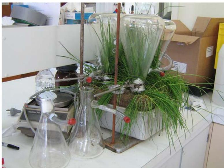
Figure 2: Laboratory set up to monitor N<sub>2</sub>O emissions from intact leaves of pasture plants.
