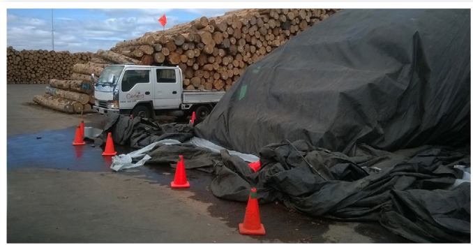
Methyl bromide fumigation of logs at Tauranga port
