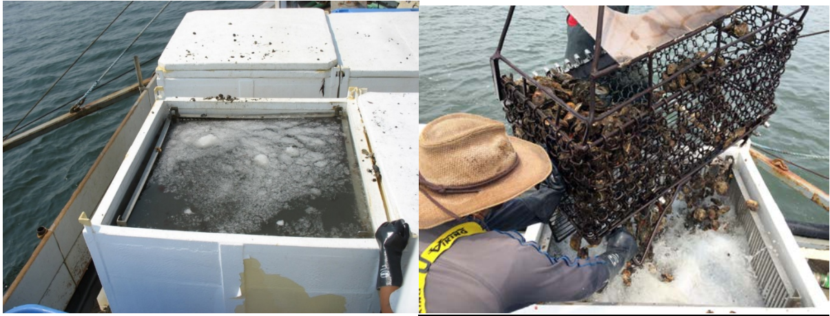
Figure 2 & 3: Photos of ice water slurry systems on harvesting vessels
