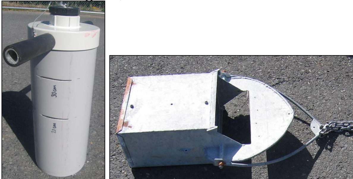
Figure 4: Large hand corer (left) and anchor box dredge (right) for sampling
