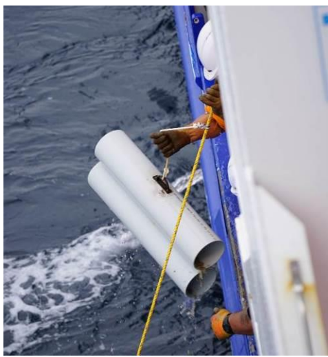
Figure 6: PVC octopus pot design (top-left), configuration along the mother line (top-right, taken from FINS 1980) and photograph of pot unit being retrieved during the survey (bottom).
