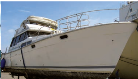
Moderately fouled hull – needs a clean. Fouling organisms already present and fertile ground for marine pests to take hold.
