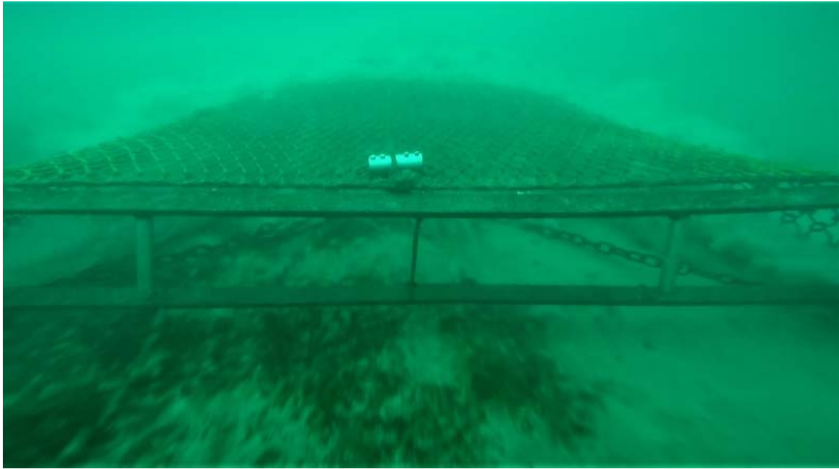
Figure 7: GoPro video frame grab showing survey ring-bag dredge during a tow, Marlborough Sounds, May 2019. Note the metal housing containing the depth logger is attached to the top of the dredge.
