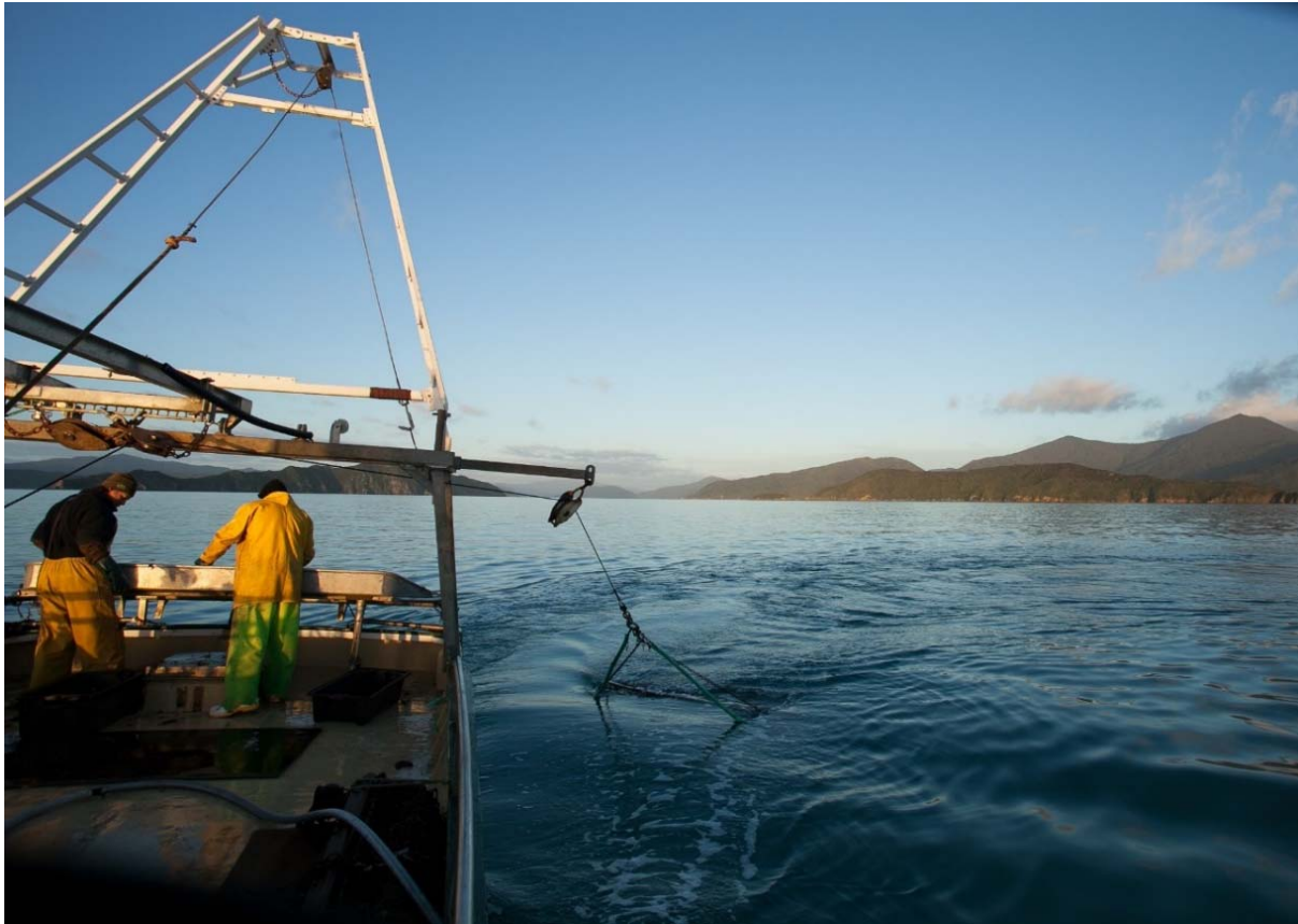
Figure 3: Stern of FV Okarito showing deployment of ring-bag dredge in Marlborough Sounds (May 2014 survey). Photo credit: J. Williams.
