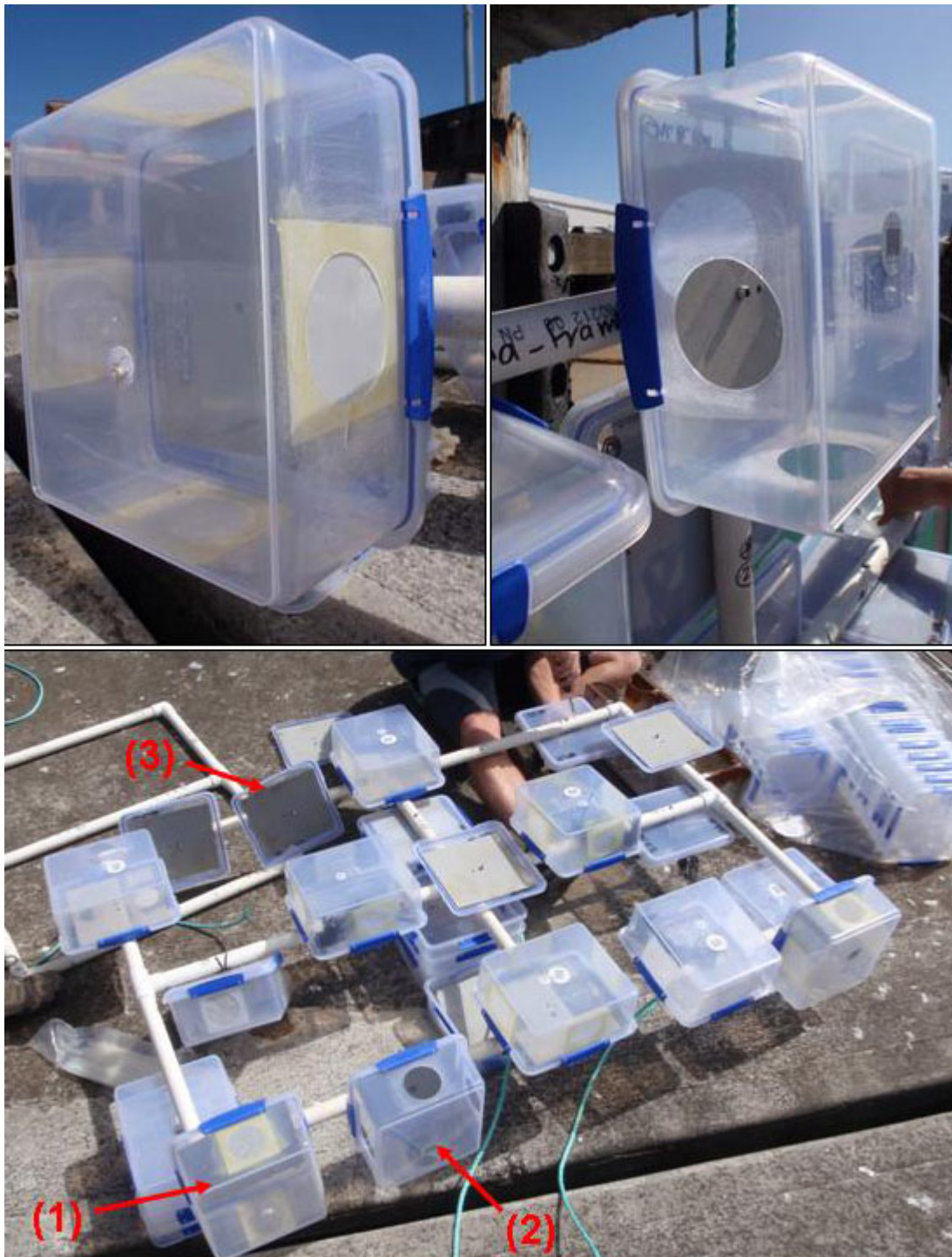
Figure 3: The experimental chambers. Top row: images of settlement chambers with (left) and without (right) mesh walls enabling water and oxygen exchange. Bottom: PVC settlement frame carrying enclosures with plankton mesh windows (1), without plankton mesh windows (2) and settlement surfaces without enclosures (3).
