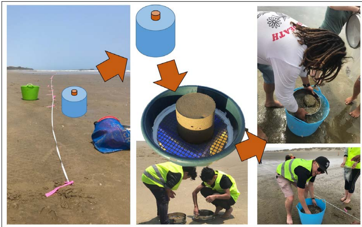
Figure 8: Series of photographs illustrating the process of collecting and then sieving of sediment cores.
