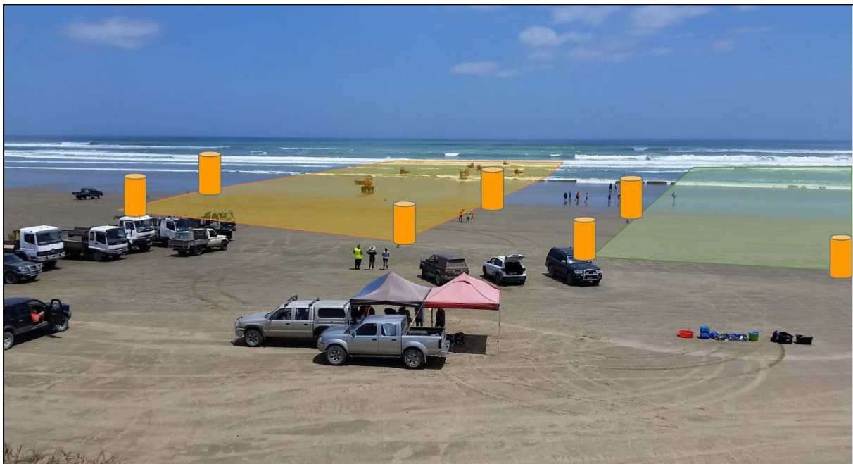
Figure 4: Experimental set up at Hukatere showing impact (orange) and control (green) zones. Loaders can be seen entering and exiting the surf in the impact zone.
